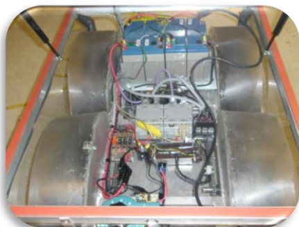
Figure 3: JΩtron's Electrical System
